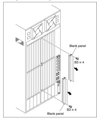
Insert the desired board into the corresponding slot and tighten the two screws (with drop-safe) of the each board.
